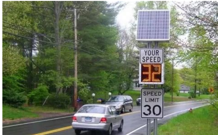
This driver feedback signs lets drivers know the speed they are traveling and can tell them to slow down.
